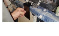
17. Cut and solder new wires to the factory washer motor wiring as an extension. Fit blade crimps to the end ready to connect to the new pump. NOTE: Green is the positive wire in the factory wiring.
