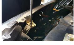
5. Next, remove the bolts securing the top of the bumper
